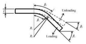
Fig 1-: Springback Effect in L Bending [12]
