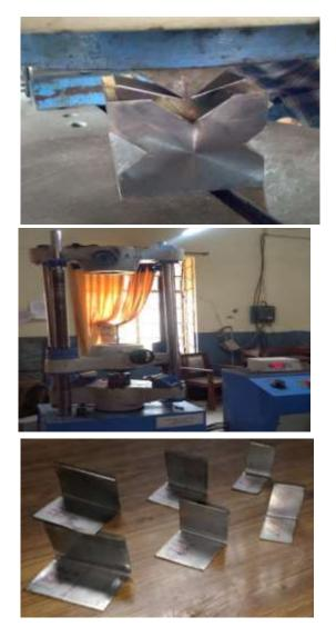
Fig 2-: Experimental setup, Die & punch, and Bent sample
