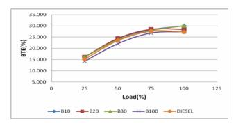
Fig -4: Variation of brake thermal efficiency with load
