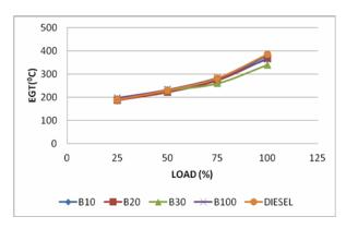
Fig -5: Load v/s Exhaust gas temperature
