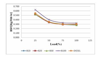
Fig -3: Variation of brake specific fuel consumption with load
