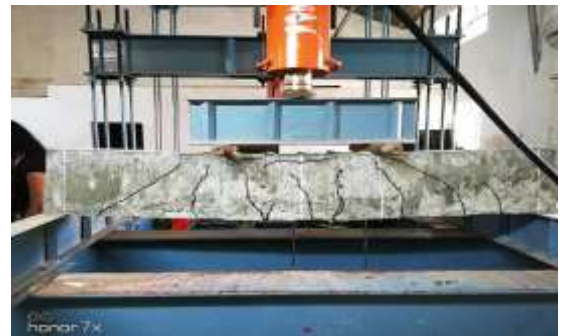
Fig -8 Crack pattern of control beam
