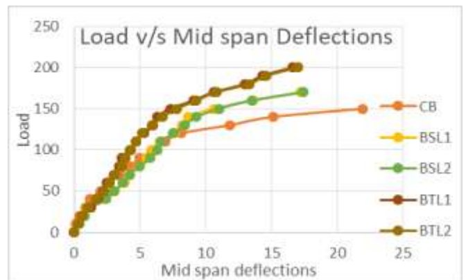
Fig -9: the load v/s mid span deflections of the beams
