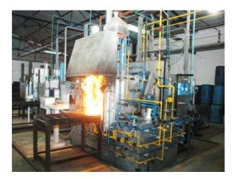
Fig- 2: Sealed Quench Furnace
