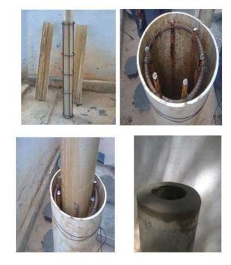
Figure 1: Casting Process
