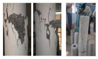
Figure 4: Failure pattern for Conventional Column
