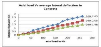
Figure 11: Axial load Vs average lateral deflection in Concrete
