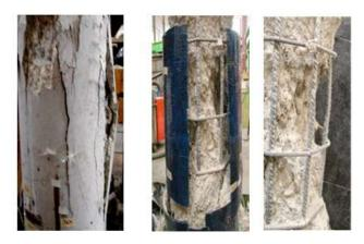
Figure 5: Failure pattern for Solid Column
