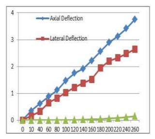
Figure 7: Load and Deflection Behavior of Solid RCC Column
