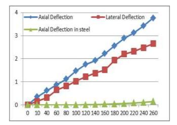
Figure 8: Load and Deflection Behavior of Hollow RCC Column
