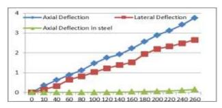
Figure 9: Load and Deflection Behavior of Conventional Hollow RCC Column confined with External FRP Jacketing
