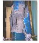
Figure 6: Failure pattern for Hollow FRP Column
