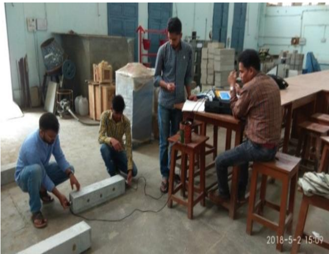
Fig -5: Ultra-sonic Pulse Velocity Test being conducted on GGBS-PQC and MS-PQC specimens
