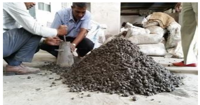
Fig -2: Slump Test
