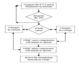
Fig -4: Flow chart for the analysis of compensation of reactive power
