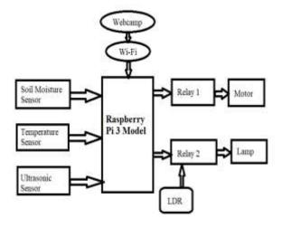
Fig 1: Irrigation Control System (Transmitting Section)
