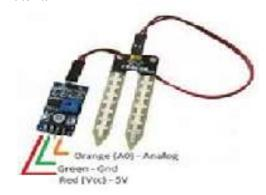
Fig 3.2.1: Soil Moisture Sensor
