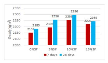
Fig.5 Graph showing density of cubes cured at 90°c in oven
