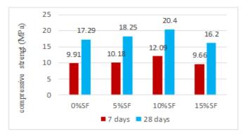
Fig.1 Graph showing compressive Strength (MPa) cured at 90°c in oven
