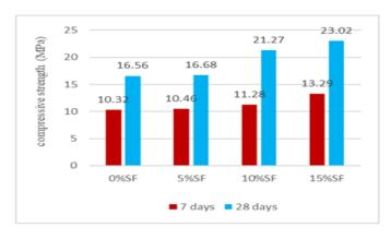
Fig.2 Graph showing compressive strength (MPa) cured at 150°c in oven
