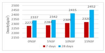
Fig.6 Graph showing density of cubes cured at 150°c in oven
