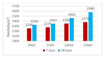
Fig.8 Graph showing density of cylinders cured at 150°c in oven
