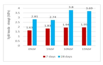
Fig.4 Graph showing Split tensile Strength (MPa) cured at 150°c in oven.
