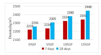
Fig.7 Graph showing density of cylinders cured at 90°c in oven
