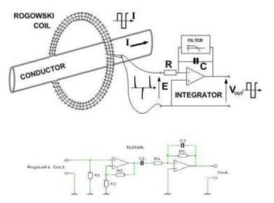
The coil is made up of a coaxial cable. Copper is wounded on it which is then shortened at other end so that the current will return to same position. And then 2 wires are taken out which is then connected to opamp circuit. When current starts flowing it generates magnetic field and this magnetic field when interacted with rogowiski coil induces emf by faradays law of electromagnetic induction. This induced emf is then applied to the opamp circuit.
