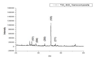
Fig.3 (b) X-Ray Diffractogram of TiO2-SiO2 Nanocomposite
