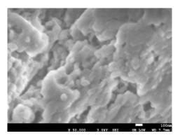
Fig.4(a) FESEM image of TiO<sub>2</sub> nanoparticle
