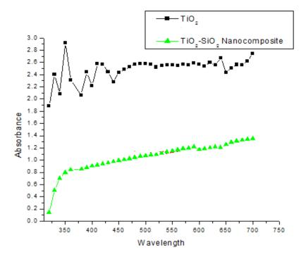
Fig -1 Absorbance spectra of TiO<sub>2</sub> and TiO<sub>2</sub>-SiO<sub>2</sub> nanocomposite
