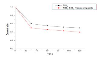
Fig -2 (c): Concentration vs Time plot of degraded dye solution with  $TiO_2$  and  $TiO_2$ -SiO<sub>2</sub>
