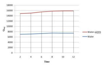
From the above graph we concluded that: With increases the time the average heat transfer rate also increases. Nanofluid gives better heat transfer than water.
