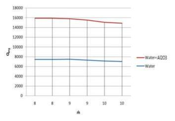
From the above graph we concluded that: From graph we see as we decreases the mass flow rate, there is average heat transfer rate of the nanofluid increases. In the graph shows average heat transfer of the nanofluid is greater than water. 4. Time (min) Vs. Average heat transfer rate (W)
