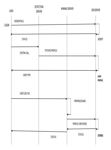
Fig -2: Process of DIIAS Framework
