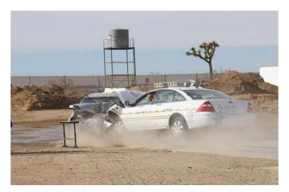
Figure 3: NHTSA research crash test carried on two Ford 500.
