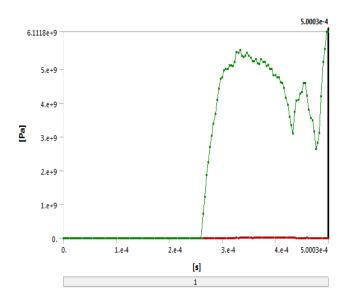
Chart-3: Equivalent stress graph of Pressure vs. time at 100 m/s
