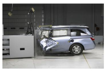
Figure 1: Frontal crash test carried for Honda Odyssey 2012.
