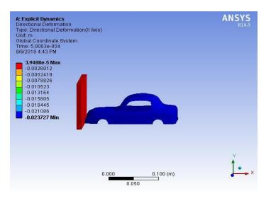
Fig-7: Directional deformation at 100 m/s
