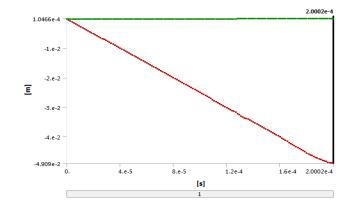
**Chart-5**: Directional deformation graph of deformation vs. time at 250 m/s
