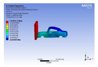
Fig-8: Directional deformation at 250 m/s
