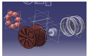
Fig. 6: Exploded view of planetary ball power transmitting system
