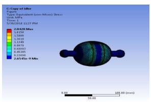
Fig. 10: Fixed equivalent stress.
