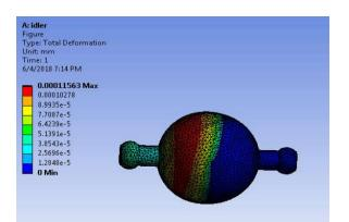
Fig. 7: total deformation of planetary ball when torque is high
