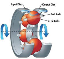
Fig. 1: working of planetary ball continuously variable transmission system
