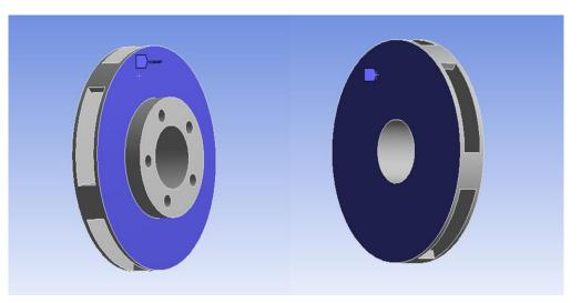
Figure- 4: (a)Heat flow on the first surface, (b)Heat flow on the second surface
