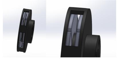
Figure- 7: Installation of TEGs on the inner sides of the disc
