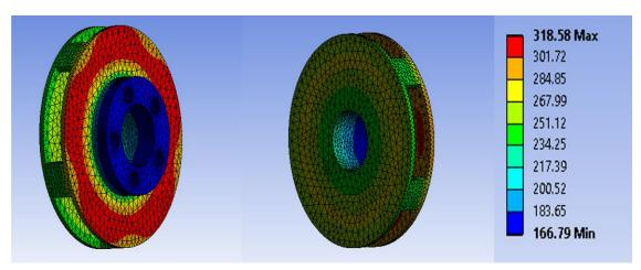
Figure- 6: Temperatures of different zones in a disc
