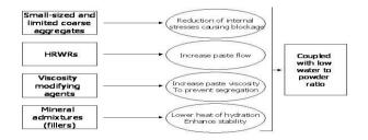
Fig -1: Principles of SCC Mixture Design
