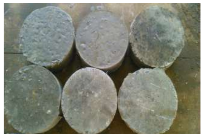
Figure15 Test Specimen with 0.75% of Crimped Fibre
