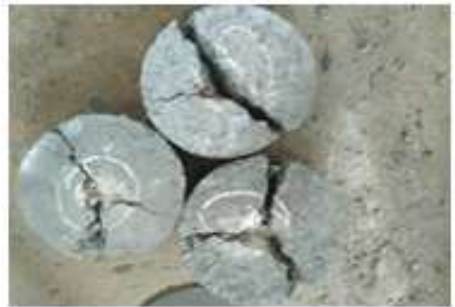
Figure 21 Final Crack of 0.75% Crimped Fibre @ 28 Days
