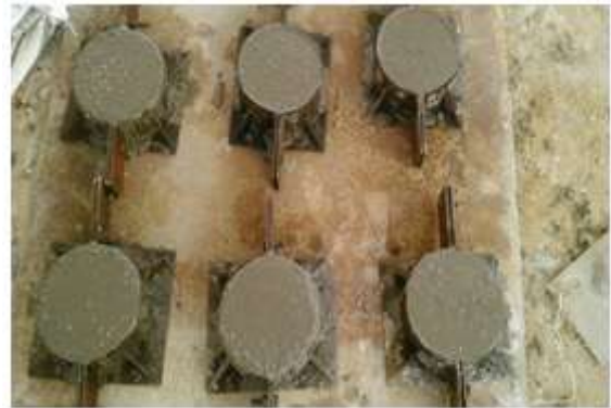
Figure13 Test Specimen in impact mould
