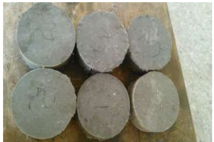
Figure14 Test Specimen with 0.5% of Crimped Fiber
