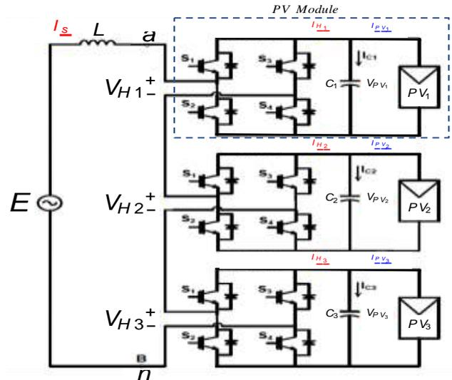
Figure1: Grid connected 7-level CHB PV converter
