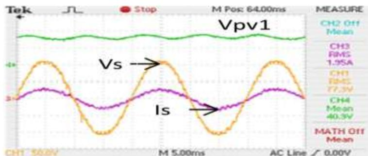
**Figure18:** Injected current into the grid and voltage of the arrays under modified MPPT during asymmetrical condition
