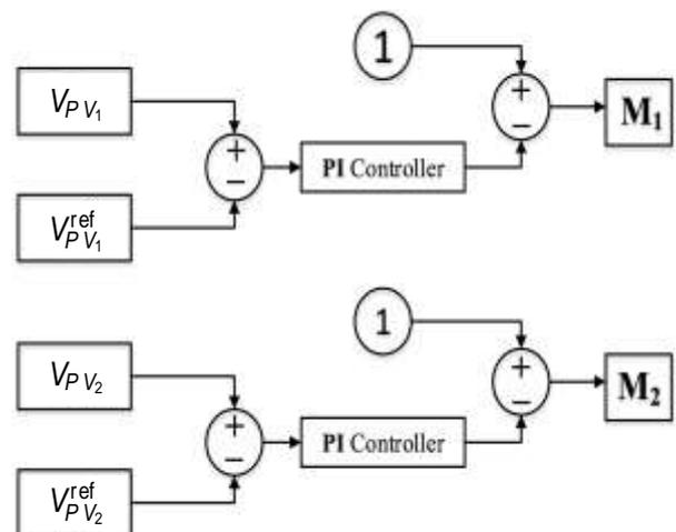
Figure4: Utilization coefficients controller
