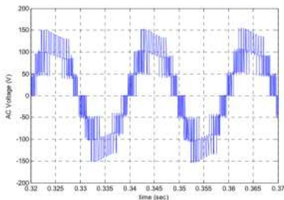
**Figure9:** AC-side voltage of 7-levels CHB inverter under modified MPPT during asymmetrical condition
