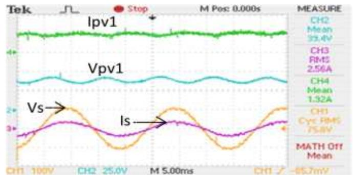
Figure13: Injected current into the grid, voltage of the grid, voltage and current of one PV cell during symmetrical condition
