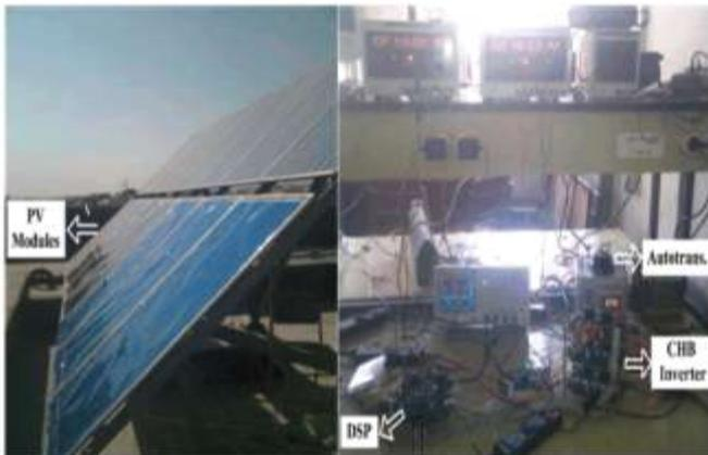
Figure12: Experimental set up to validate the simulation results
