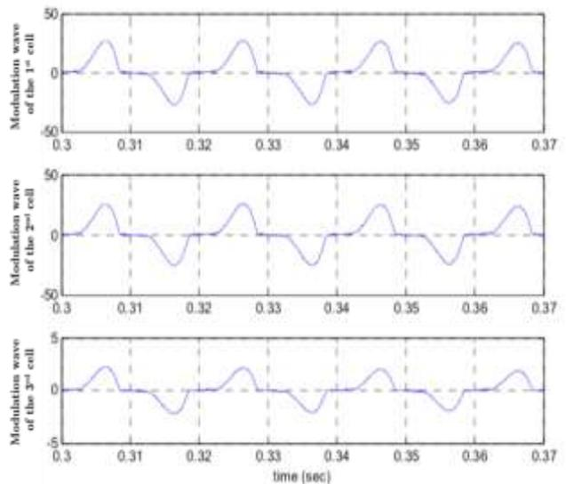
**Figure10:** Modulation wave of the three cells under normal MPPT during asymmetrical condition
