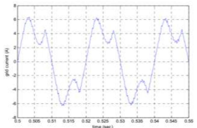
Figure6: Injected current to the grid under normal MPPT during asymmetrical condition
