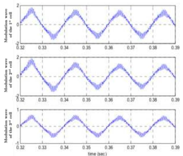
**Figure11:** Modulation wave of the three cells under modified MPPT during asymmetrical condition
