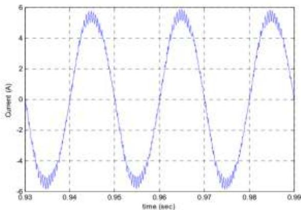
**Figure7:** Injected current to the grid under modified MPPT during asymmetrical condition
