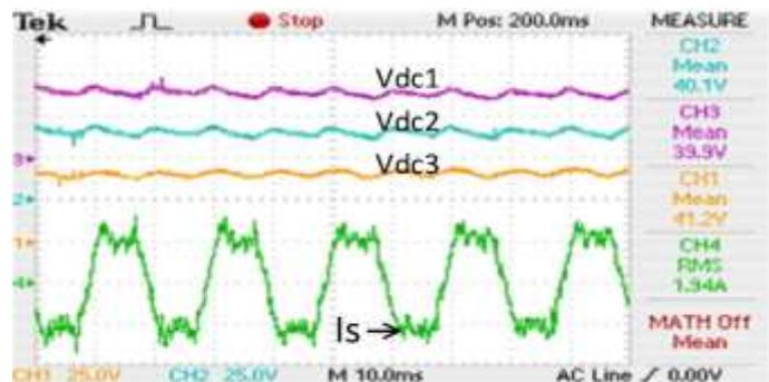
Figure14: Injected current into the grid and voltage of the arrays under normal MPPT during asymmetrical condition
