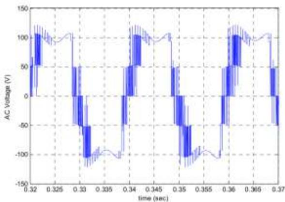
**Figure8:** AC-side voltage of 7-levels CHB inverter under normal MPPT during asymmetrical condition
