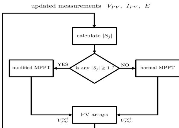
Figure2: Overview of the voltage controller
