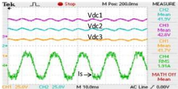
**Figure15:** Injected current into the grid and voltage of the arrays under modified MPPT during asymmetrical condition
