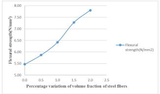
Figure 4: Variation of flexural strength due to percentage variation of steel fibers for M-Sand optimized SCC
