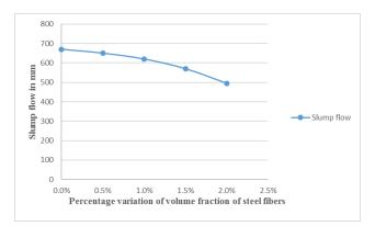
Figure 1: Slump flow for percentage variation of volume fraction of steel fibers
