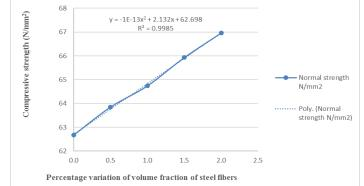
Figure 5: Best fit curve for compressive strength
