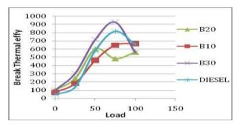
Chart- 5: Comparison of Load Vs Brake thermal efficiency for different blends of algae oil.
