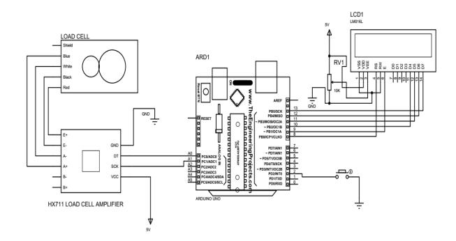
Fig. 3: Circuit diagram for the developed system
