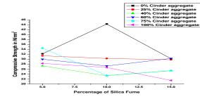
**Fig-1:** Compressive strength with different percentages of cinder aggregate with different percentages of silica fume
