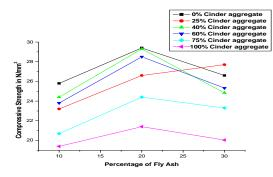
Fig-2: Compressive strength with different percentages of cinder aggregate with different percentages of fly ash
