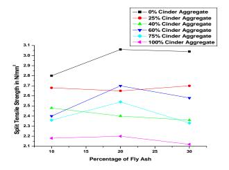
**Fig-4:** Split Tensile strength with different percentages of cinder aggregate with different percentages of fly ash
