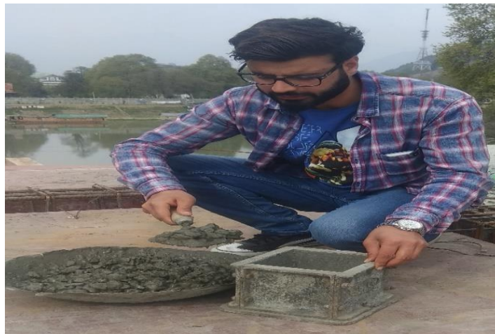
Figure 8. Filling cube of pervious Concrete
