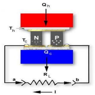
Figure 6 Electricity Generation With One Thermoelectric Power Module [15]
