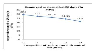
Figure 4.3: Compressive strength of percentage rate of ceramic replacement at 28 days.
