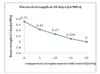
Figure 4.6: Flexural strength of percentage rate of ceramic replacement at 28 days.
