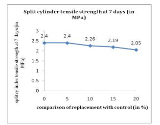
Figure 4.7: Split cylinder strength test of percentage rate of ceramic waste used at 7 days.
