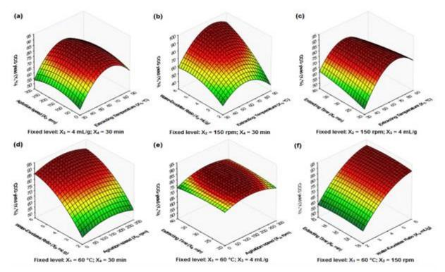
**Fig -1:** Response surface showing the effect of extracting temperature and agitation speed (a), extracting temperature and water to exudates ratio (b), extracting temperature and extracting time (c), agitation speed and water to exudates ratio (d), agitation speed and extracting time (e), and water to exudates ratio and extracting time (f) on the Crude Cashew Gum (CCG) extraction yield.
