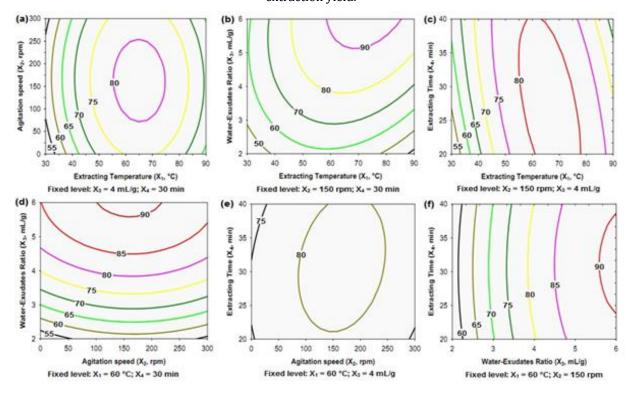
Fig -2: Contour plot showing the effect of extracting temperature and agitation speed (a), extracting temperature and water to exudates ratio (b), extracting temperature and extracting time (c), agitation speed and water to exudates ratio (d), agitation speed and extracting time (e), and water to exudates ratio and extracting time (f) on the Crude Cashew Gum (CCG) extraction yield.
