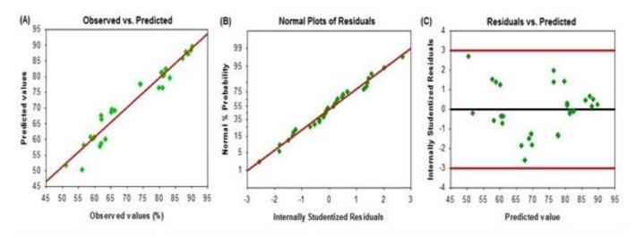
Fig -3: (A) Predicted response versus actual value, (B) Normal probability of internally studentized residuals and (C) Plot of internally studentized residuals vs. predicted response for model adequacy checking.
