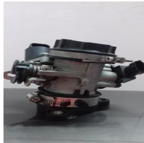
Fig -1: Throttle body of KTM RC 390
