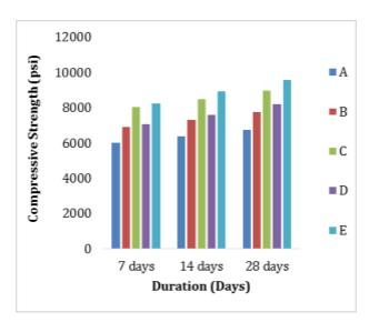
**Chart -1**: Compressive Strength Test Results of Five Different Mixtures
