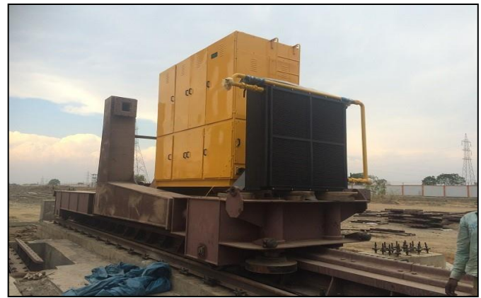
Figure-14: Side arm charger with drive & Hydraulic power pack Assembly
