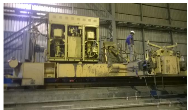
Figure-15: Side arm charger in operation at site
