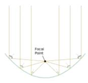
Fig -2: A diagram of a parabolic trough solar collector
