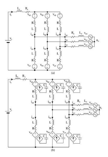
**Fig. 4.** Models of the M<sup>2</sup>C. (a) Considering the arms as voltage sources. (b) Considering switching effects and capacitor dynamics.
