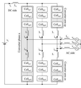
Fig2. DC/Three-phase modular multilevel converter circuit topology
