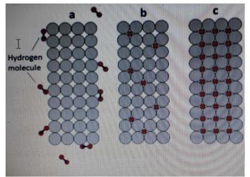
Figure (3): Chemical adsorption mechanism. [29]
