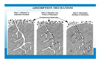
**Figure (1):** Steps of adsorption mechanism, (1) diffusion of adsorbate to adsorbent surface (2) Adsorbent migrate in to the pores (3) Monolayer buildup of Adsorbate [53]
