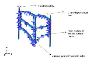
Fig-3: Fine mesh of bridge joint seal enlarged
