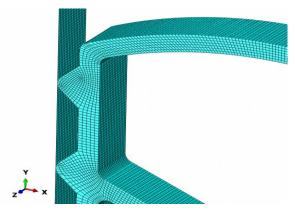
Fig-4: FEM of Bridge joint seal with loads and boundary condition
