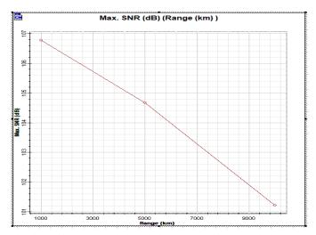
The SNR vs range graphs for both the techniques are depicted above which gives us the result that OFDM system's SNR value is the higher from the polarization technique and bears a good value of SNR at three different points of range i.e on 1000km, 5000km and 10,000 km.
