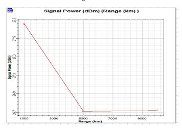
As we can see easily from the first graphical report that the value of received power is very less in polarization interleaving as compared to OFDM. Which is highest 27.7 at 1000km and drops to 26.7 at 5000km.
