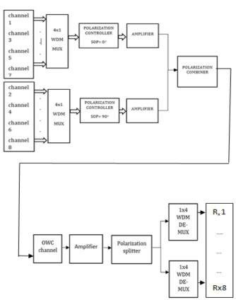
Fig.2 Block diagram of Is-OWC WDM system with polarization-interleaving
