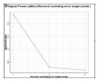
The above two graphs show the system efficiency when they are subjected to some values of pointing errors. The lowest value of received power in OFDM system is 46dbm with 3 micro radian pointing error. Whereas in Polarization interleaving it is 25dbm at 3 micro radian pointing error.
