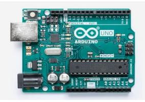
Figure 1: Arduino Uno microcontroller **4.2 OpenCV/python**
