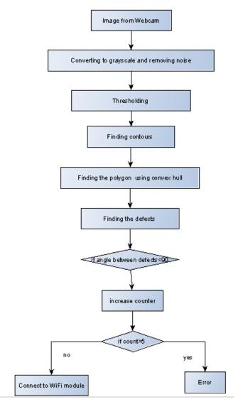
Figure 9: Process Flowchart for hand gesture extraction
