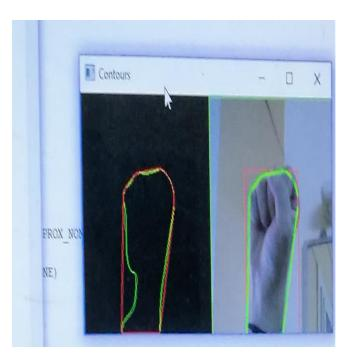
Figure 10: Detecting 5 defects in the hand gesture.
