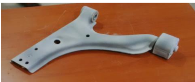
Figure 3 Lower suspension arm during blue light scanning Points generated from blue light scanning is transferred to CatiaV5. Model is created using surfaces. The model looks as below in CatiaV5
