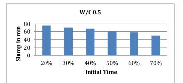
**Fig 1:** Variation of slump with initial Time
