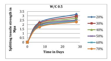
Fig 3: Variation of splitting tensile strength with flaky aggregate percentage
