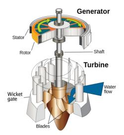
(Fig.1.3 .1 vertical axis hydraulic turbine)
