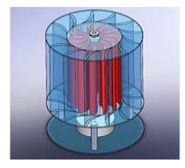
(Fig 1.2.1 vertical wind mill)
