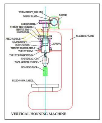
Fig. 2. Portable Vertical Honing Machine
