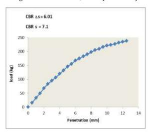
Fig.13: CBR Test Result, Case C (4 days of soaking)
