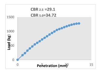
Fig.10: CBR Test result, Case B (Un-soaked)
