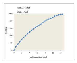
Fig.14: CBR Test Result, Case D (Un-soaked)
