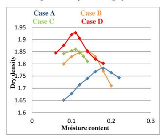
Fig.5: Modified proctor test comparison graph
