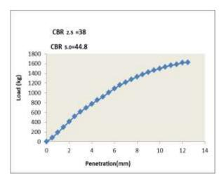
Fig.12: CBR Test Result, Case C (Un-soaked)
