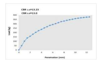
Fig.8: CBR Test Result, Case A (Un-soaked)
