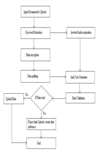
Fig -1: System flow diagram
