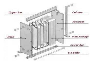
Fig.1 Exploded view of PHE
