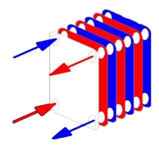
Fig.7 Plate and frame PHE
