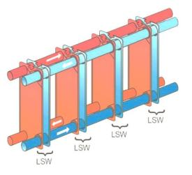
Fig.6 Semi-welded PHE
