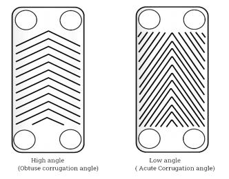
Fig.2 A typical plate of a PHE
