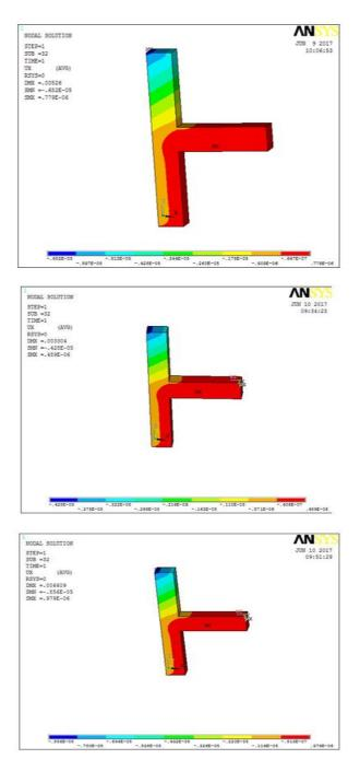
Figure :3 :Deformation of T jointfor5,10,15,20 KN
