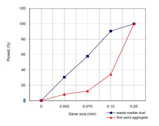
Fig. -1. Grain size distribution of fine sand aggregate and marble dust.
