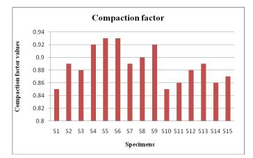
Graph No.4.3 - Results of Compaction Factor test for all specimens
