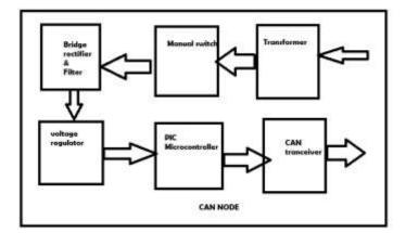
Fig5.Block Diagram of CAN node
