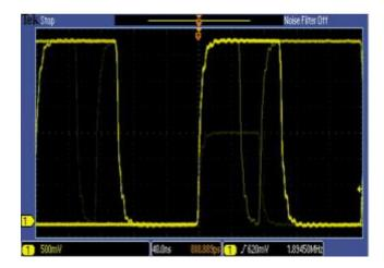
Fig7.CAN bus signal on Tektronix Oscilloscope
