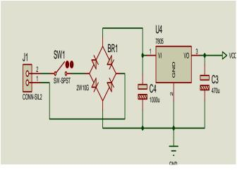
Fig3. Circuit diagram of power supply
