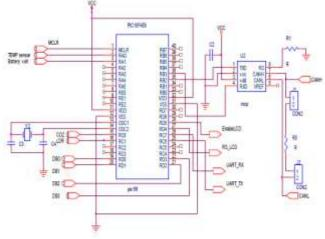
Fig7.Interfacing of PIC microcontroller with MCP 2551
