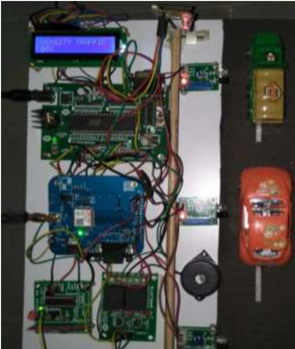
Fig -6: IR-2 Sensor detected when the traffic is Medium Traffic Density
