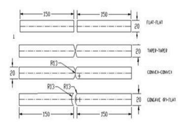
Figure 3.21: Interface geometry combinations for FW
