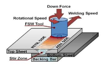
Figure 1.1: Schematic drawing of friction stir welding
