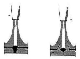
Figure.2 DCSP TIG and DCRP TIG weld formation
