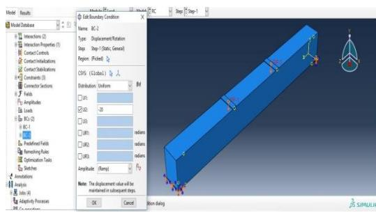
**Fig - 10 : Boundary conditions in ABAQUS**
