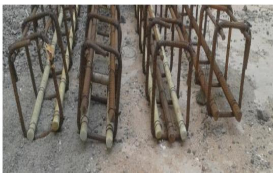
**Fig - 5 : Reinforcement cage**
