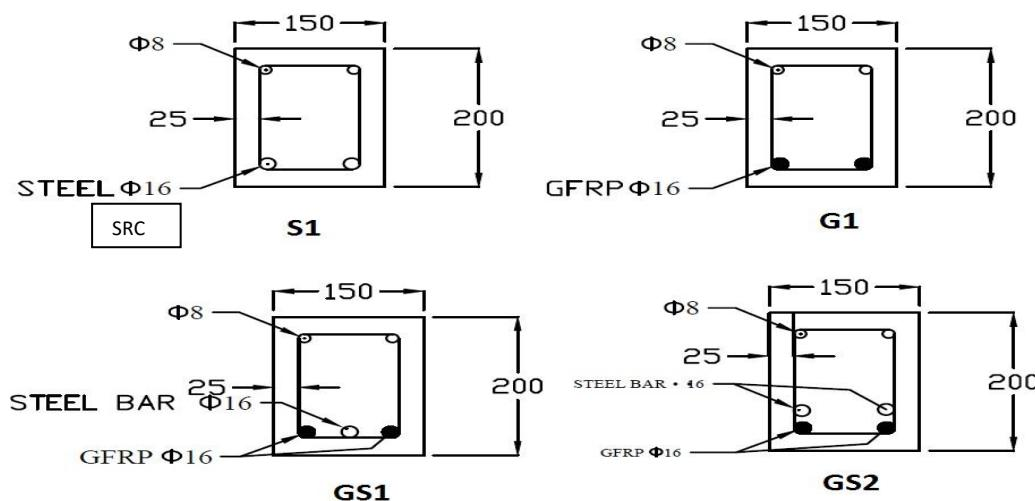
**Fig - 3 : Description of beams cross section**
