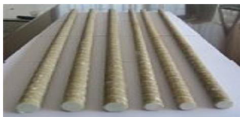
**Fig - 1 GFRP Rebar**
