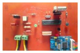
Fig-3: Board for temperature sensor with CAN and AVR interfacing
